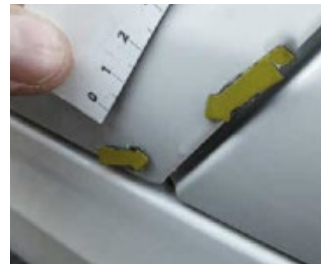
Poor paint job, with paint dripping (if painted through a non-authorized repairer).
