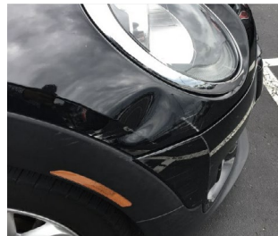
Greater than 20mm diameter or paint surface penetration.
